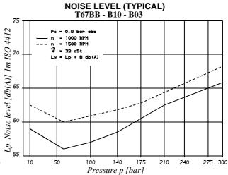
Double pump noise level is given with each section discharging at the pressure noted on the curve.
