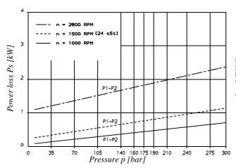
Total hydromechanical power loss is the sum of each section at its operating conditions.
