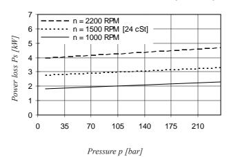
Total hydromechanical power loss is the sum of each section at its operating conditions.
